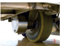
The stainless propulsor motor manages aggressive and wet environments
